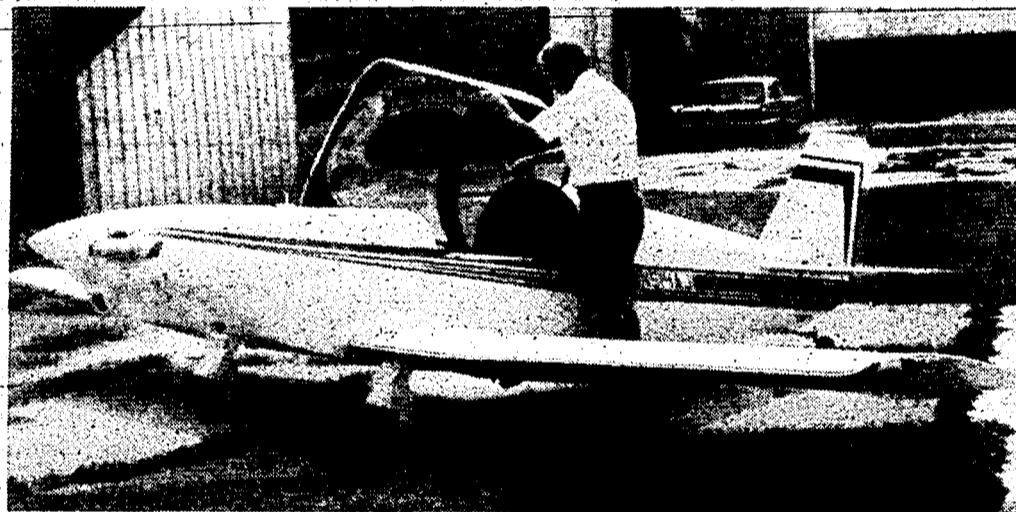
NOW COMPLETED, the plane is in full flying trim. Moore hand-built everything on the aircraft except the plastic cockpit bubble and wheel castings. After a three-hour maiden flight, Moore reported no problems. In flight, the wheels retract for better aerodynamics. Most of last winter was spent preparing the exterior for painting. Moore says the plane's skin is so smooth that dust just blows off.
